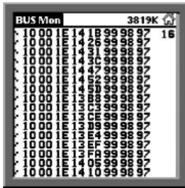
Figure 4.15 Bus Monitor Screen with All IDs Filtered Except for ID $10
